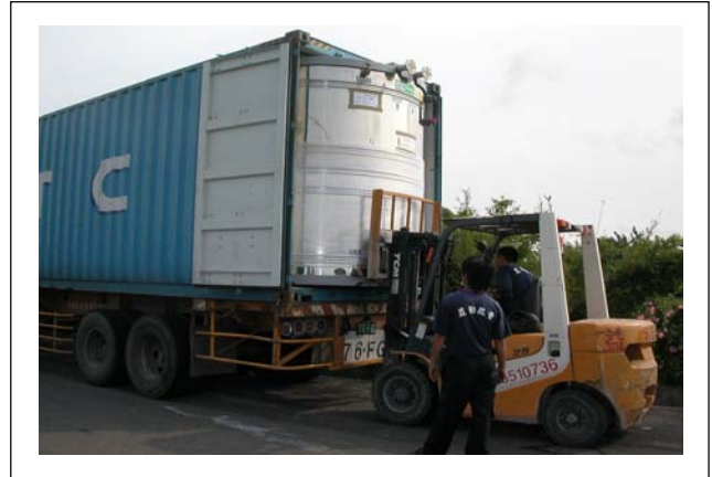
儲冰槽貨櫃運輸 Ice storage tanks transported by container truck
